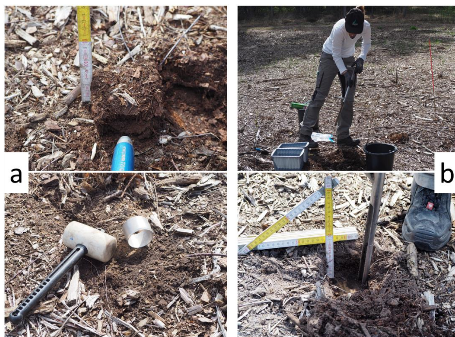
Figure 8 Soil sampling devices: a) humus/top soil (0-5 cm) sample: spatula/trowel (above) or sampling ring (below); b) sub soil (5-30 cm) sample: push probe
