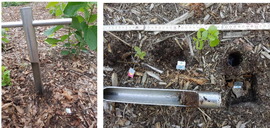
Figure 9 Burying of tea bags with a soil corer
